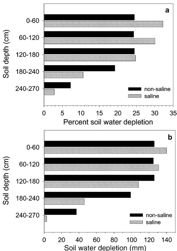
Fig. 6. Relative (a), and absolute (b) soil water depletion by depth over the entire safflower growing season in saline and non-saline conditions. Effective salinity of saline plots ( $n = 7$ ) averaged  $7.2 \text{ dS m}^{-1}$  and that of non-saline plots ( $n = 6$ ) averaged  $2.1 \text{ dS m}^{-1}$ .
