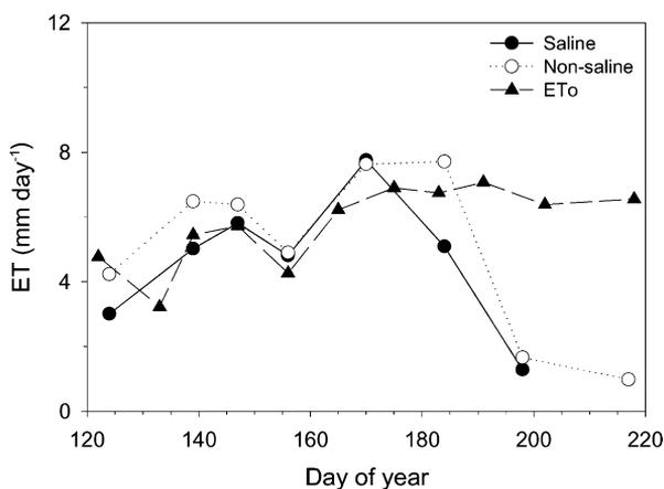
Fig. 3. Reference ( $ET_0$ ) and crop ( $ET_c$ ) evapotranspiration of safflower grown in non-saline ( $EC_e = 2.1 \text{ dS m}^{-1}$ ) and saline ( $EC_e = 7.2 \text{ dS m}^{-1}$ ) soil.  $ET_0$  is derived from a CIMIS weather station located at the experimental site.  $ET_c$  was calculated from soil water depletion measured using a sealed-source neutron hydroprobe.
