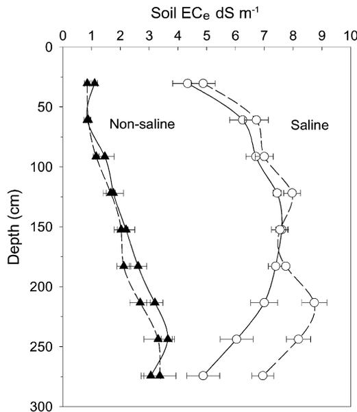
Fig. 1. Averaged pre-plant (—) and post-harvest (---) soil  $EC_e$  with depth (0–2.7 m) for saline (○) and non-saline (▲) plots irrigated with either saline or non-saline water. Effective  $EC_e$  at pre-plant and post-harvest is 6.5 and 7.3  $dS\ m^{-1}$  and 2.2 and 2.0  $dS\ m^{-1}$  for saline and non-saline plots, respectively. Error bars are S.E.,  $n = 7$  for saline and  $n = 6$  for non-saline treatments.
