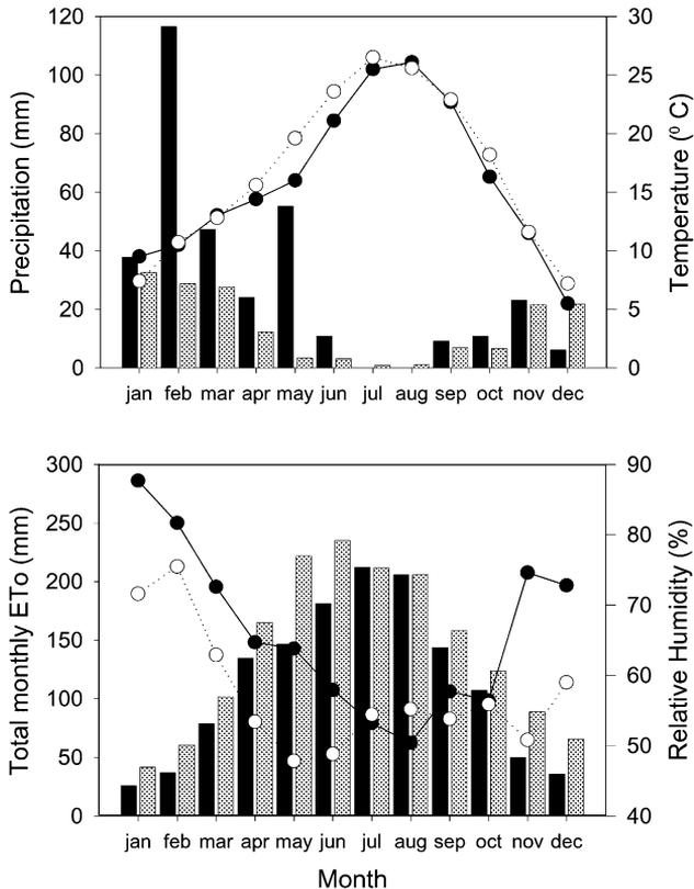
Fig. 2. Total monthly precipitation,  $ET_o$ , average temperature and relative humidity for 1998 and long-term averages obtained from CIMIS. Bars represent precipitation (upper) and total  $ET_o$  (lower). Lines are for temperature (upper) and relative humidity (lower). Black bars and solid lines represent 1998 data. Shaded bars and broken lines represent long-term averages.
